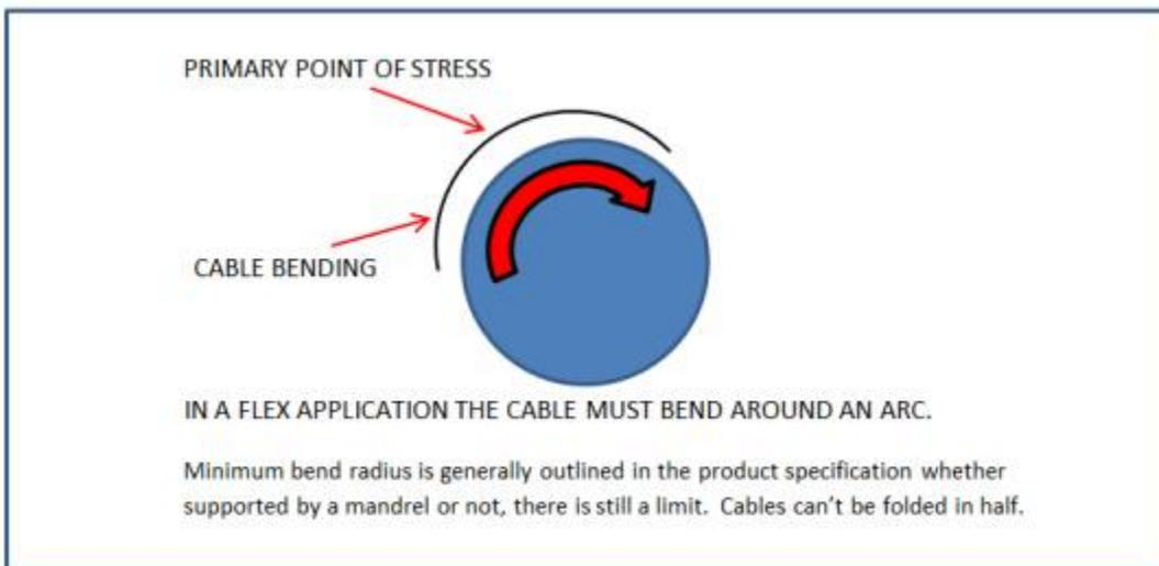
As shown above, when a cable flexes, it bends around an arc. Let's examine what's happening. The larger the arc around the center point, the greater the distance. Take a look at the illustration of the target below.
