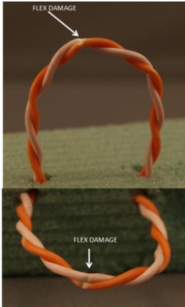
PHOTO 2 & 3: PHOTO OF BONDED PAIR AFTER LIMITED FLEXING. THIS SAMPLE WAS NOT FLEXED TO FAILURE BECAUSE IT CONVEYS THE ISSUE CLEARER AS IT BEGINS TO BREAK DOWN. NOTICE THE "WORK HARDENING" OF THE CONDUCTOR INSULATION AT THE TOP OF THE ARC. THE CABLE HAS CREASED AND NOW ALL BEND FORCES ARE BEGINNING TO CONCENTRATE IN AT THE ONE WEAK POINT. EVENTUALLY THIS WILL BECOME THE POINT OF FAILURE.
