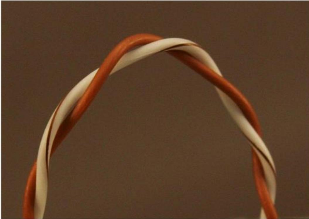
PHOTO 1: UN-BONDED PAIR BEING BENT IN AN ARC. NOTICE THE CONDUCTOR TO CONDUCTOR SEPARATION IS MINIMAL EVEN THOUGH THE PAIRS ARE NOT BONDED TOGETHER.
